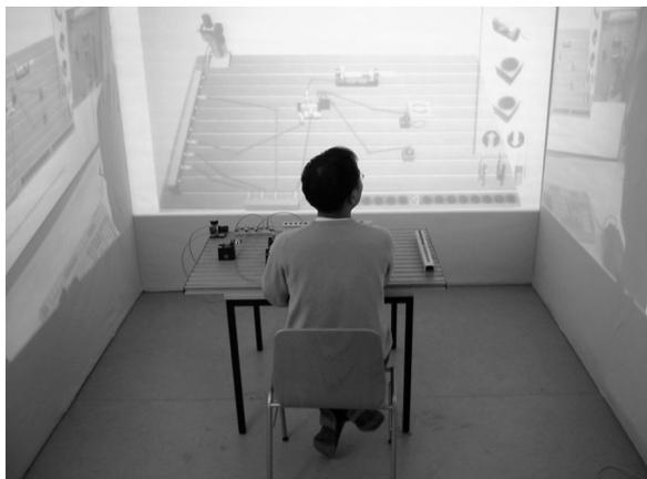
Figure 2. Workspace using CAVEs with the real workbench (center), the virtual one in front and the remote counterparts (left and right pane)
