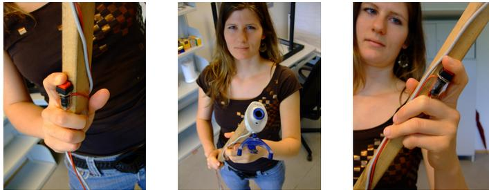
Figure 2: *Gun cam*, with fire button (left) and reload button (right)
