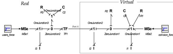
Fig. 4: Traditional bond graph model of ball manipulator (not considered the haptic interface)
