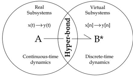
Fig. 1: The concept of mixed reality bond graph modeling
