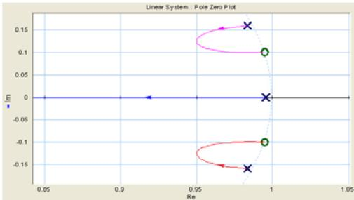
Fig. 9 : Root locus of the unity feedback system that has the forward transfer function  $G_{forward}$
