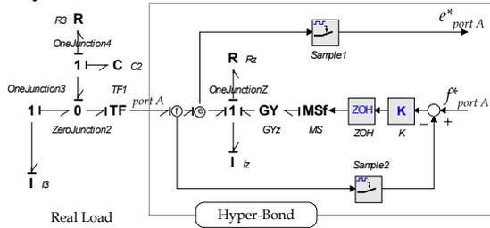
Fig. 8: Hyper-bond subsystem for the haptic interface
