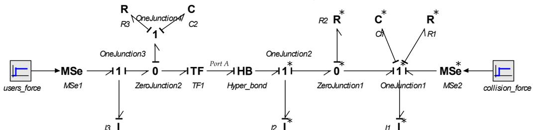
Fig. 6 : Mixed reality bond graph modeling of the haptic ball manipulator
