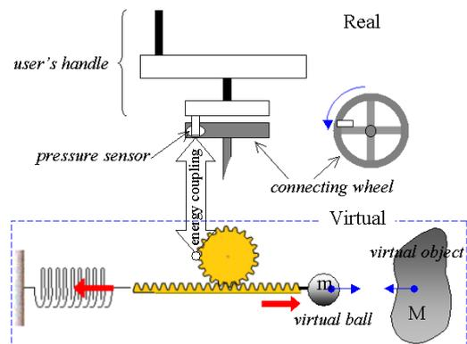
Fig. 3: Structure of haptic ball manipulator
