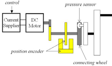
Fig. 7 : Sketch of hardware parts of the hyper-bond subsystem.
