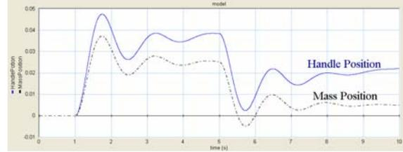
Fig. 10 : Behaviors of handle (I3) position and mass (I1) position when the system has  $G_{forward}$  such as Eq. 6 and its  $K$  is 1060.
