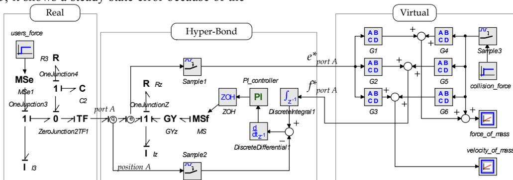
Fig. 12: Implementation of the mixed reality bond graph modeling of Fig. 6 in 20-sim
