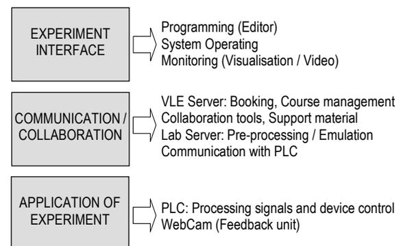
Fig. 2. Architecture of the remote PLC experimentation lab kit
