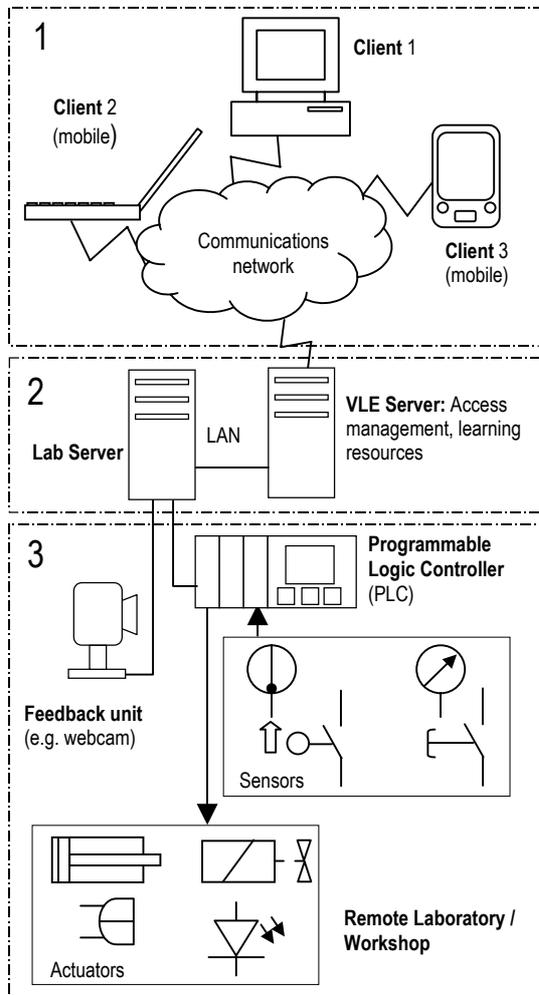
Fig. 3. Schematic presentation of the remote PLC experimentation lab kit
