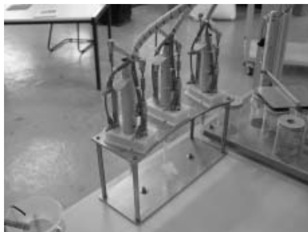
Fig. 5: Pneumatic system for dispensing liquids using pipettes, Source Chemicals (right)
