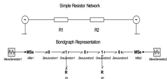
Fig. 4: Resistor Network in Bond-graph Representation (MSe = modulated source of effort)
