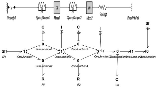
Fig. 9: Two-Mass Spring-Damping System (Example 4.11)
