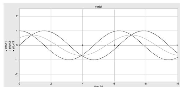
Fig. 5: Result from 20-sim simulation (...sine wave generated left, --cosine generated right, \_\_measured at the interface)
