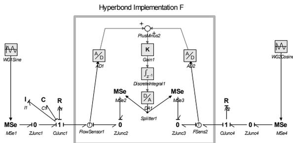
Fig. 7: Implemented Hyper-Bond for Complex System with Inductivity  $I=0.1$ , Capacity  $C=0.1$ , Resistance  $R=1.0$  and Gain  $K$
