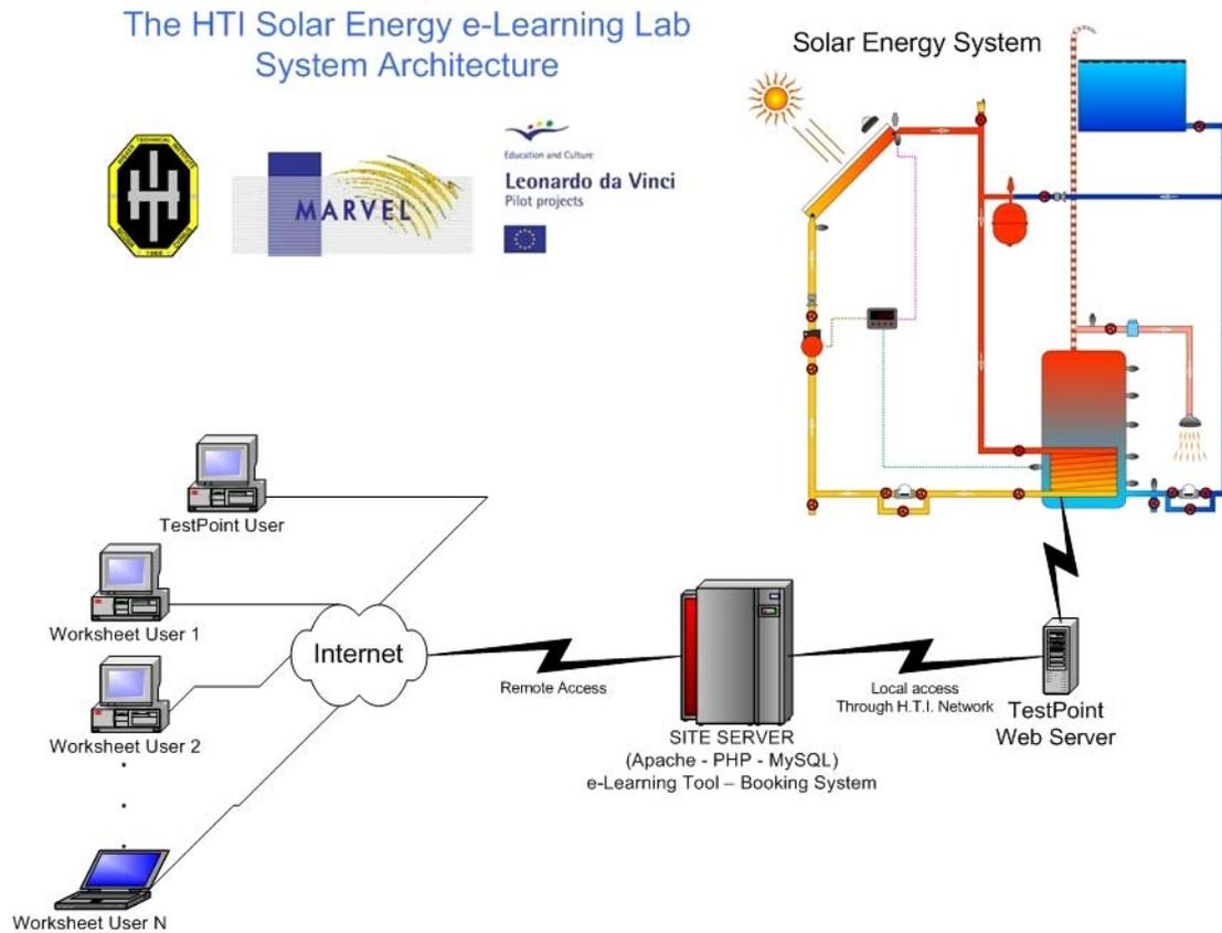
Figure 3: The System Architecture
